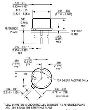
\*\*FOR SOLDER DIP LEAD FINISH, LEAD DIAMETER IS  $\frac{.016 - .024}{(0.406 - 0.610)}$
